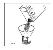
The salt container will require topping up periodically. According to the model, an indicator reminds you when filling with salt:
